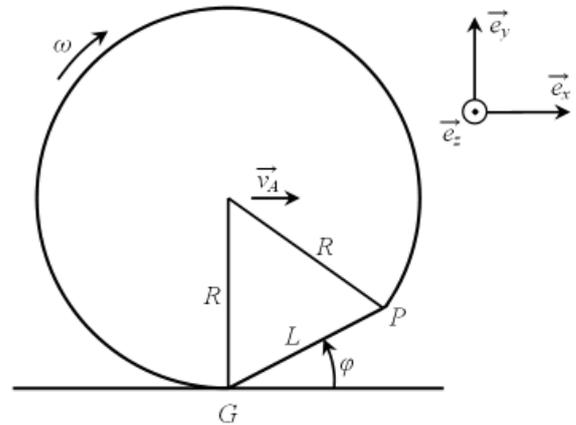
Fig.3. Geometry of a railway vehicle wheel with an idealized flat spot
