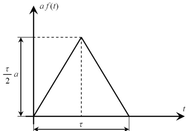
Fig.4. Transient loading of the rail
